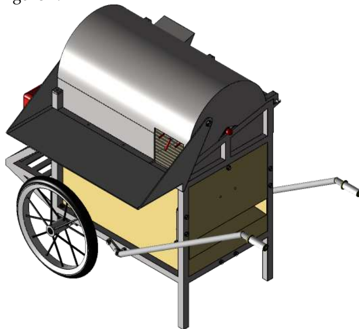
Figure 1. Rice threshing machine used for testing
