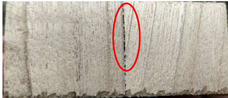
Figure 2. Thin Bond Line in Polyester Adhesive Bonding Specimens.
