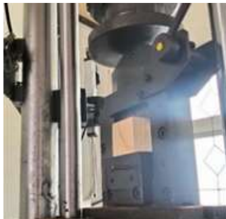
Figure 1. Bond Shear Strength Test of Sungkai Glulam Specimen.
